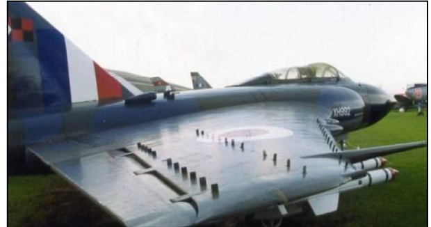
Fig. 2: VGs on RAF Javelin fighter [2]
