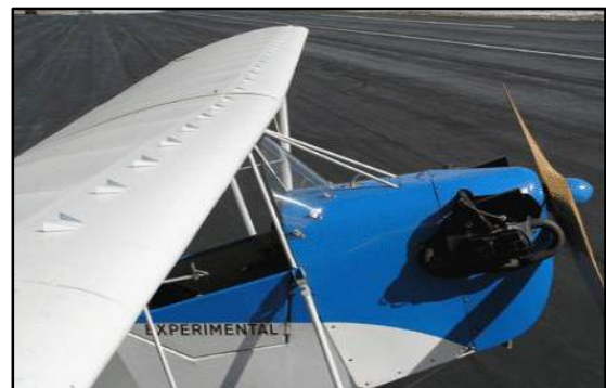
Fig. 3: VGs on Stewart Headwind aircraft [3]
