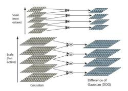
The first algorithm is to find image keypoints by computing DOG equation in different image size. The Gaussian Space equation is  $D(x,y,\sigma)=L(x,y,k\sigma)-L(x,y,\sigma)$  by k is constant of scale space of images I=(x,y)
